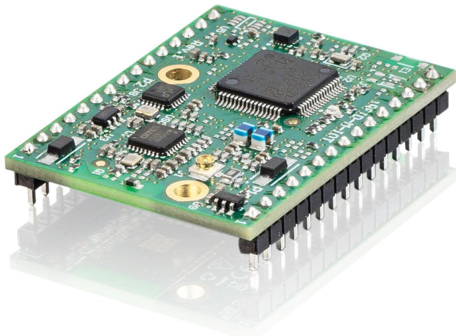
RFID HF-Reader module with WiFi and Ethernet interfaces
